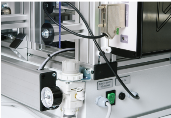
Compressed air is used for controlling web tension and compression stress level
